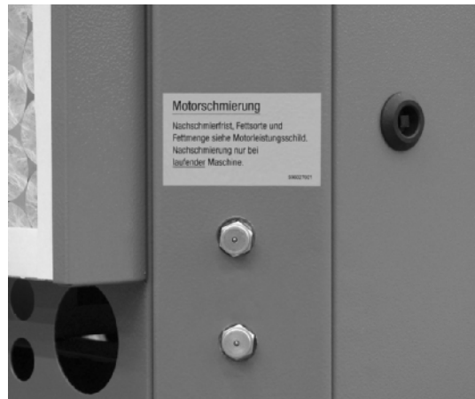
Fig. 6.13: Grease nipples of the lubricating device
